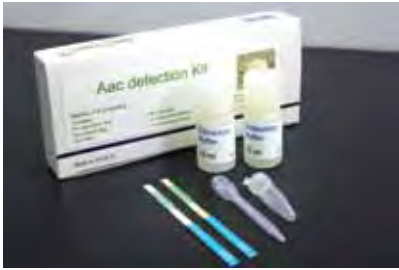
Immunochromatographic strip test for detection of Acidovorax avenae subsp. citrulli .
